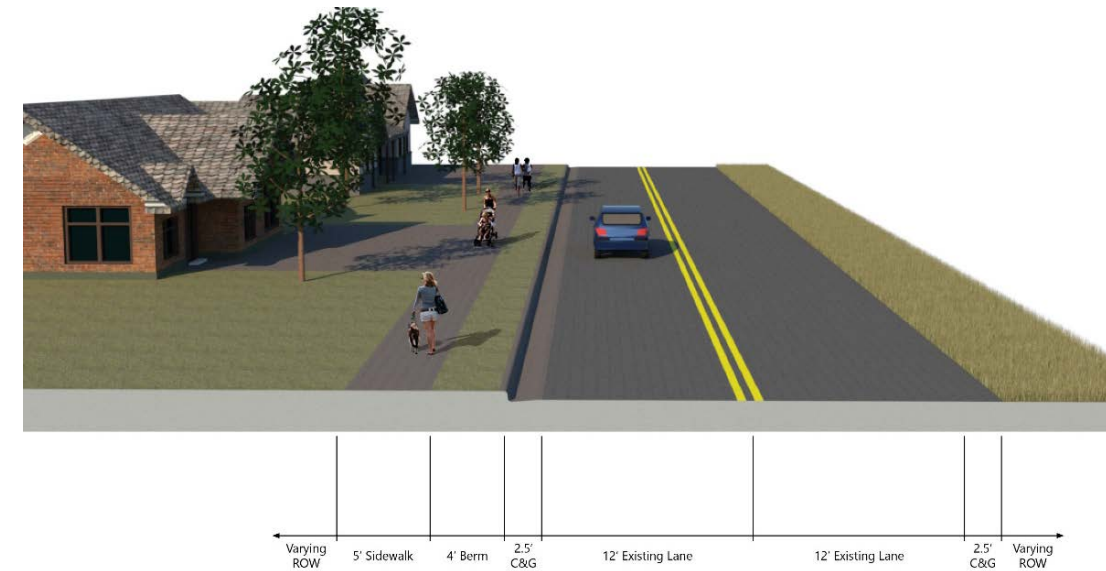
Section C – Sidewalk with Curb and Gutter
