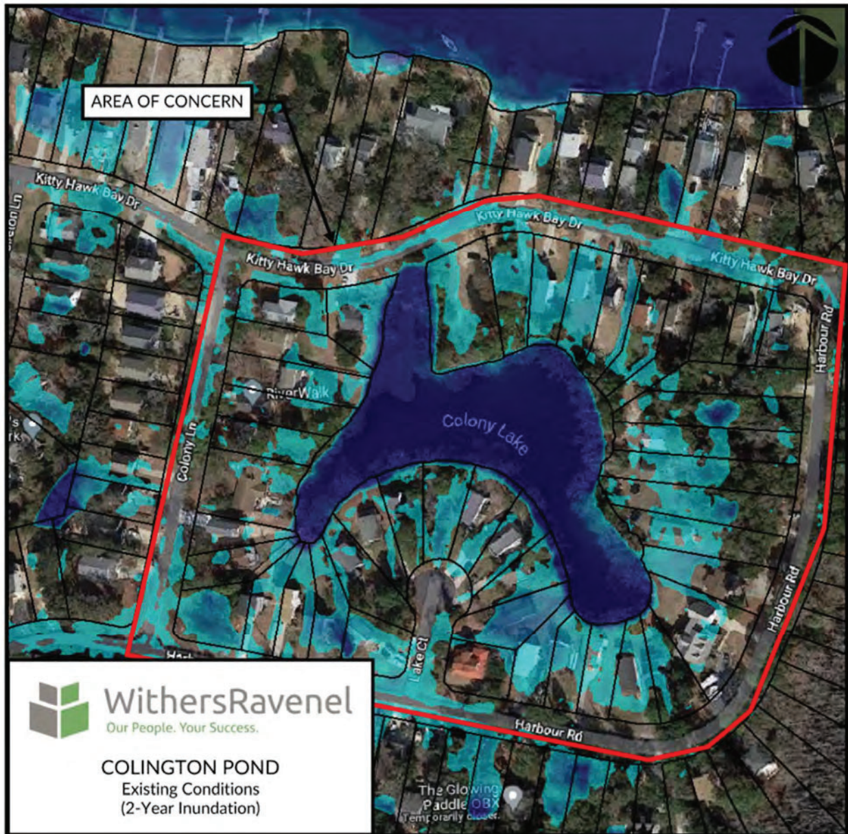
Figure 4 - Colington Pond Existing Conditions 2-Year Inundation
