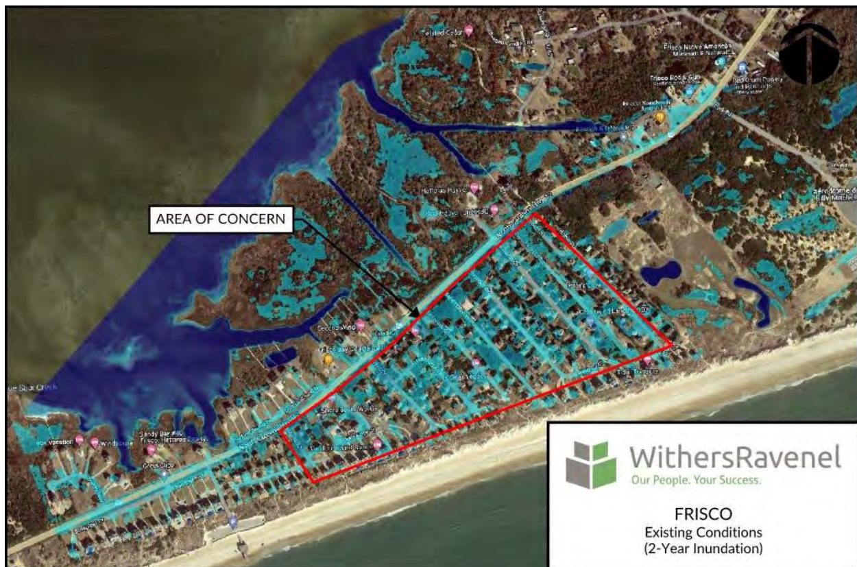
Figure 10 – Frisco Existing Conditions 2-Year Inundation
