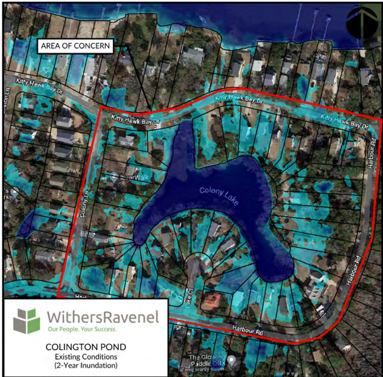
Figure 4 - Colington Pond Existing Conditions 2-Year Inundation
